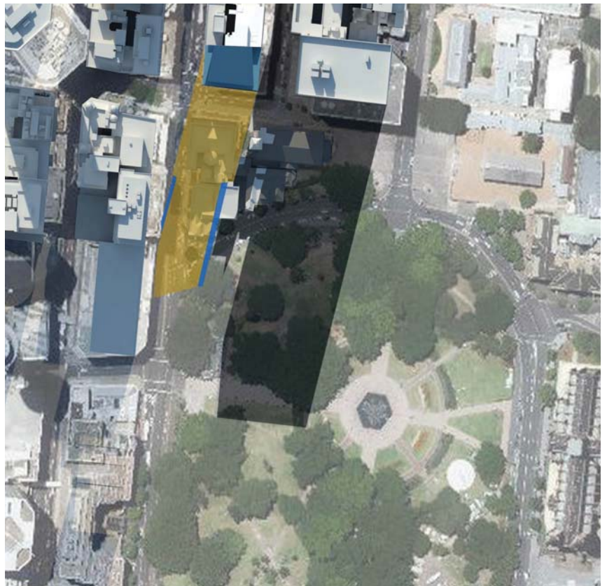
OVERSHADOWING CAST BY DCP ENVELOPE AND ADDITIONAL OVERSHADOWING CAST BY PROPOSED ENVELOPE
